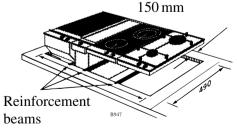
It is not necessary to attach the reinforcement beam to the work top surface, as it is held in place by a specially designed moulding, which is incorporated in the hob units flanges.
